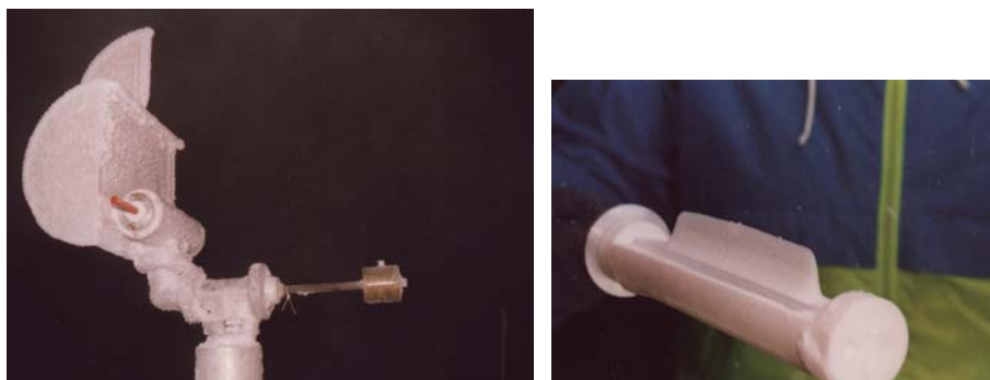
Figure 1: Cloud Water Sampling at the Sonnblick Observatory during the ALPTRAC campaigns showing the Cloud Water Sampler (Kruisz et al. 1993) and an actual sample of subcooled droplets.
